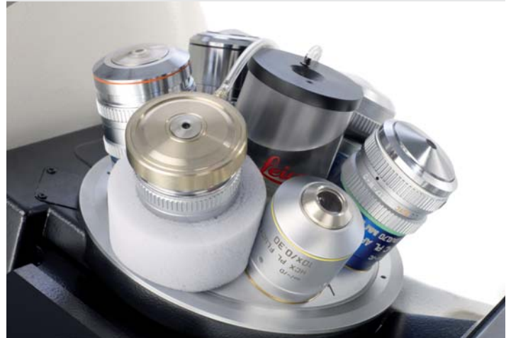
Water Immersion Micro Dispenser – Automatic supply of water immersion during experiments
